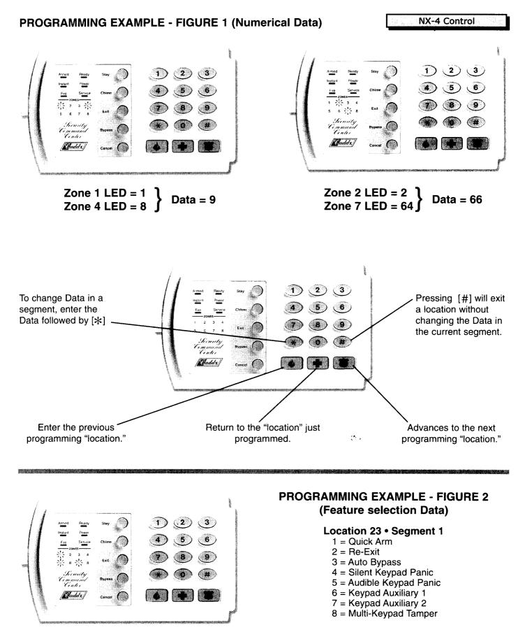
Press the key on the numeric Keypad that corresponds to the feature you wish to enable/disable. When an LED is "on" a feature is enabled, when "off" the feature is disabled. For example, with the 1, 5, & 7 LED's "on," Quick Arm, Audible Keypad Panic and Keypad Auxiliary 2 are enabled.
